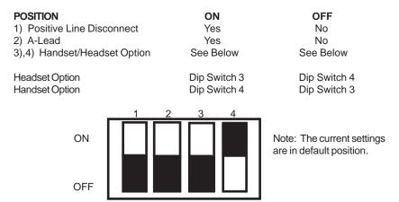
Note: Make sure the DIP switch is in default position when using handset: Position 3 Off and Position 4 On.
