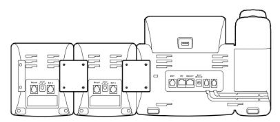
**5.** Connect the Ext jack on the host phone and the Ext in jack of the first module using one supplied cord. If you want to connect another module, connect the Ext out jack of the first module and the Ext in jack of the second module using one supplied cord. Connecting two expansion modules on a single host phone is shown as below:
