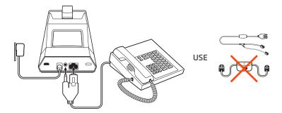
**IMPORTANT** Use configuration **A** on the bottom of the base, which works for most phones including Cisco phones.
