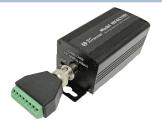
Eo2<sup>™</sup> Ethernet over 2-wire Transceiver with PoE+ Model NV-EC1701U
