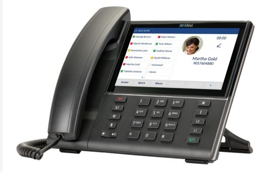
The Mitel 6873 SIP Phone is designed for power users who demand a lot from their phones. The 6873 offers executives a large 7" touchscreen display, support for today's, and tomorrow's, high speed networks through dual Gigabit Ethernet ports with embedded Bluetooth and a powered USB port for headsets. Providing remarkable HD wideband audio, an enhanced speakerphone and advanced audio processing, the Mitel 6873 SIP Phone will deliver crystal clear hands free conversations.
