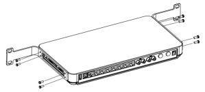
2 Push the AVHub into the rack, and then fix it to the rack with screws.
