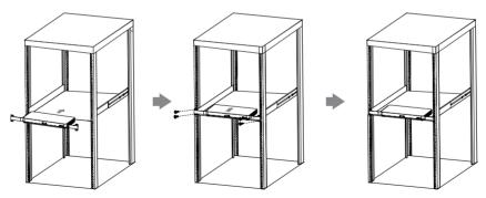
The rack in which the AVHub will be placed must be a 19-inch Rack compliant with IEC 60297. The Package Contents do not include screws.
