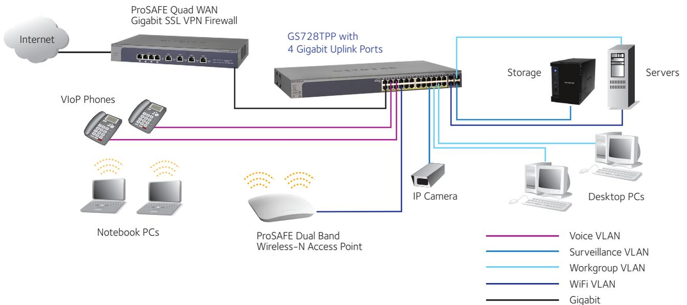
**The latest generation of Gigabit PoE/PoE+ Smart Managed Switches from NETGEAR are the right choice for the converged networks at SMBs and offer the best return on your investment.**
